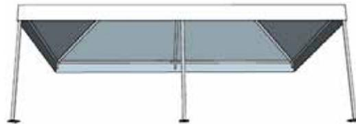
6. Lift the other side of the tent and attach the legs (with base plates). While this unit will stand on its own, it is NOT intended that the base plates be used as an anchoring method. The stakes should be driven approximately 5 feet away from the bottom of the leg. It is imperative the tent be secured with ropes and stakes or any other appropriate anchoring method. It is recommended that you do not bolt the base plates to any surface. Store the cover only when clean and dry.
