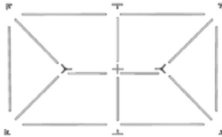
2. Start assembling the frame by inserting and pinning the Hip Rafters into the Center Crown(s). If assembling a rectangular frame insert and pin the appropriate Spreader into the Center Crown and continue to the next Ridge Top T or Center Crown. Insert and pin Rafters into the Crowns and Ridge Top T's. Insert and pin all Corner Fittings and Side T Joints to the bottom of the Hip Rafters and Rafters.
